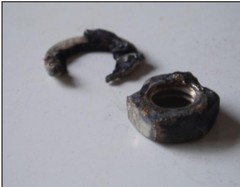
Above is the result of a loose bolt on an EV during acceleration.
